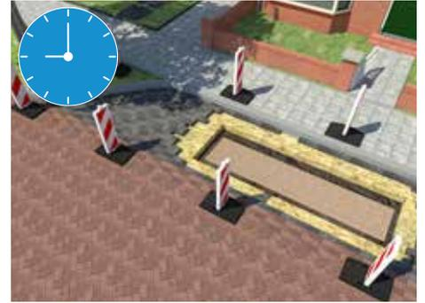
Placing water-storing package and finishing sides with drainage sand.
