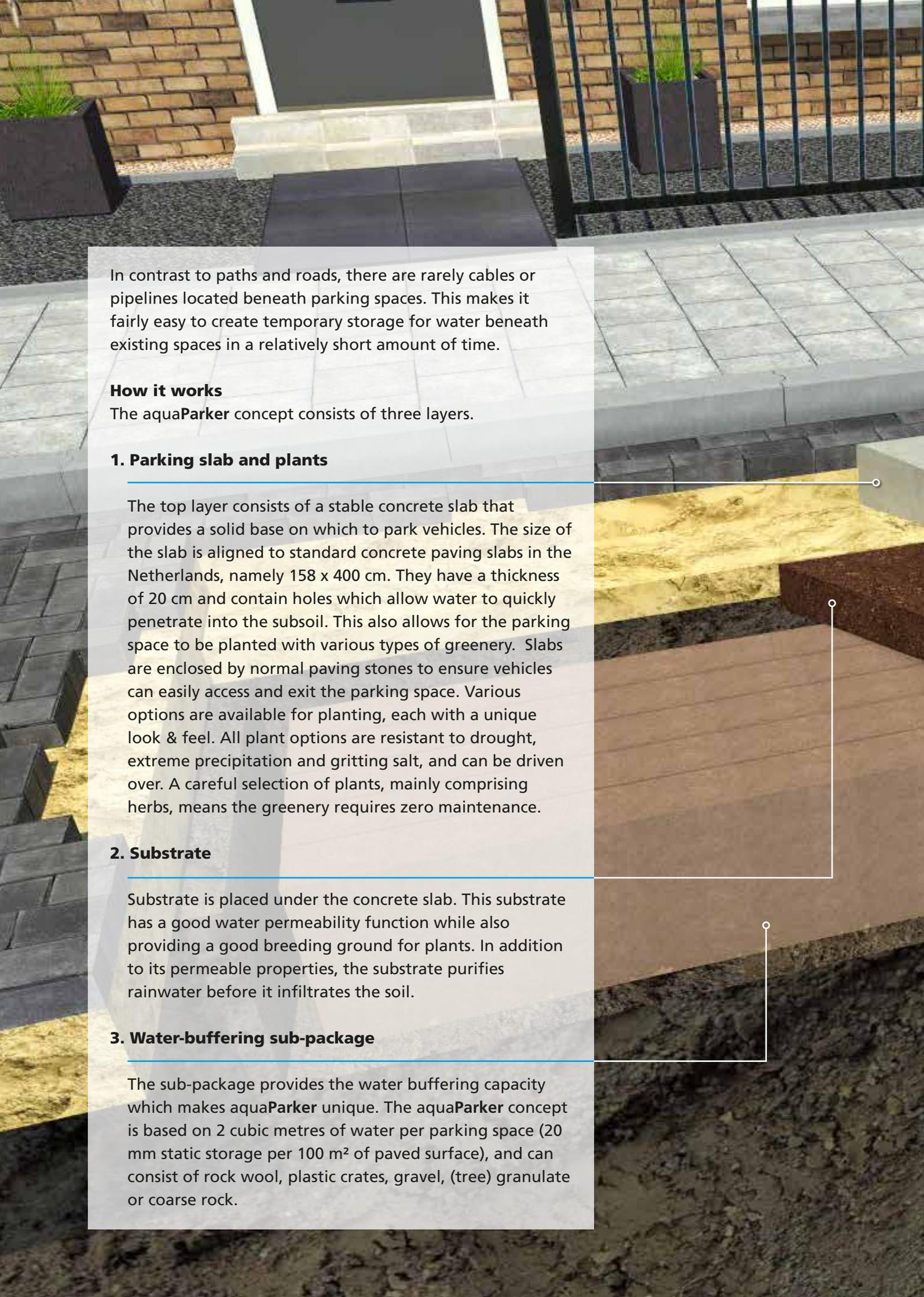
In contrast to paths and roads, there are rarely cables or pipelines located beneath parking spaces. This makes it fairly easy to create temporary storage for water beneath existing spaces in a relatively short amount of time.
